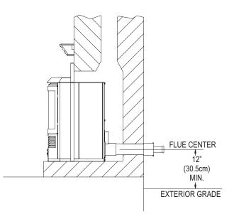
Figure 38 Minimum Exterior Grade Dimension - Existing Fireplace Installation
